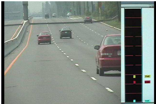
Figure 2: Video snapshot of TrafficView experiment with 3 cars on US Highway 1, in New Jersey. The left part shows the three cars on the road, while the right part shows the information displayed to the driver in the third car.
